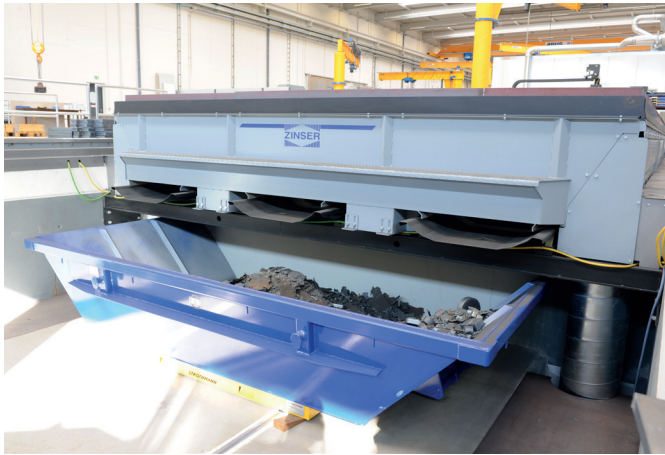
Rear view of an in-ground ZINTRAC cutting table with oscillating conveyor. Slag and scrap formed during the cutting process are removed from the cutting table via vibration chutes and transferred into the provided collection containers.
