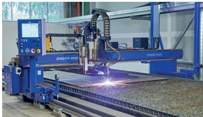
One of the two new ZINSER 4025. This machine is equipped with an oxy-fuel torch and the highly dynamic ZINSER bevel head.
